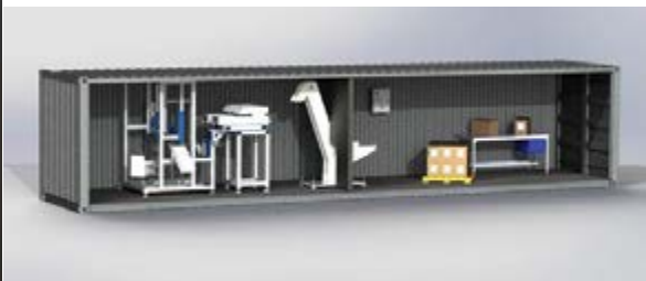
General arrangement of the automated disassembly equipment
