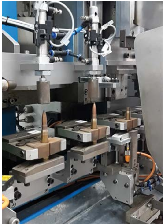
Detail view of the automated disassembly equipment
