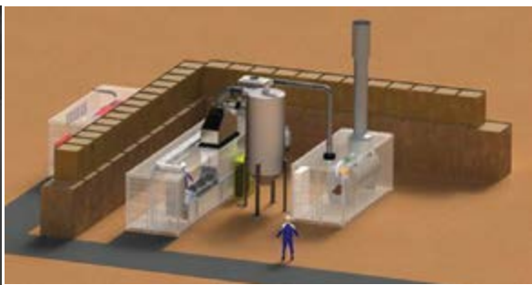
Lay-out of propellant incineration equipment with gas filtering system
